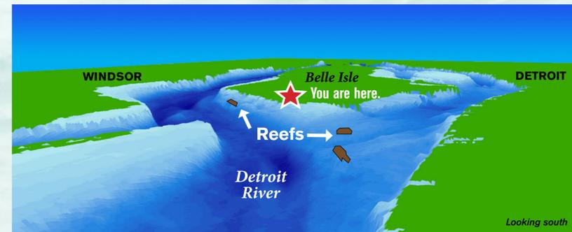
**PLANNING:** Detailed information about the river bottom and water flow are used to find the best locations for constructed reefs.
