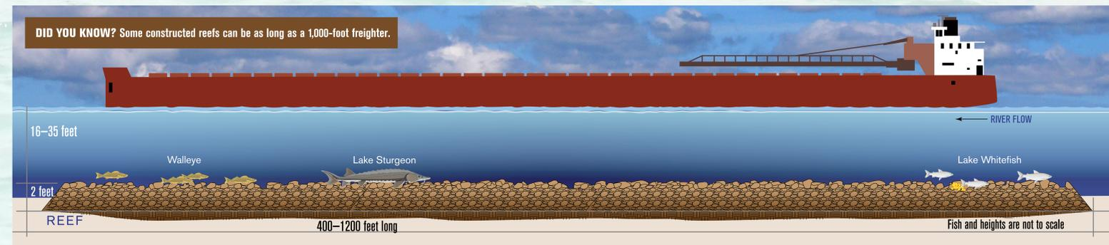
Constructed fish spawning reefs are created by placing a 2-foot layer of limestone rock rubble on the river bottom. Reefs are built in deep, fast flowing sections of the river where they will not interfere with navigation.
